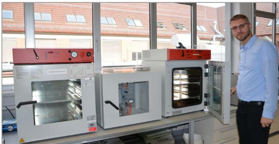
> BINDER vacuum drying chambers can be used to test granulate that will later be used in the form of implants in the human body.
