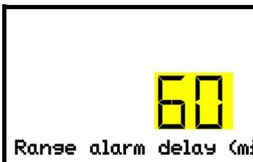
Setting the tolerance range alarm delay.
