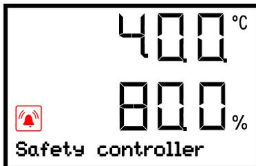
Alarm indication (example: safety controller alarm)
